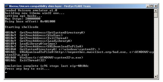
Figure 1: Initial test of the libernu Win32 environment and hooks running under Unicorn
