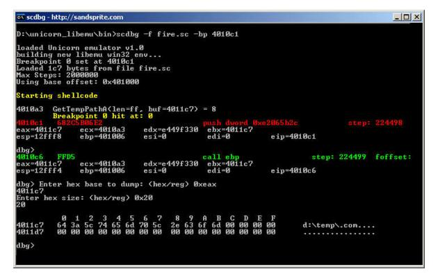
Figure 3: Imported scdbg debug shell running with Unicorn Engine and libemu shim layer
